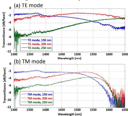
Fig. 3: Spectra for tip widths of 150, 200, 250 nm in (a) TE and (b) TM modes.
