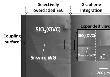
Fig. 2: Scanning electron microscope image of selective integrated part.
