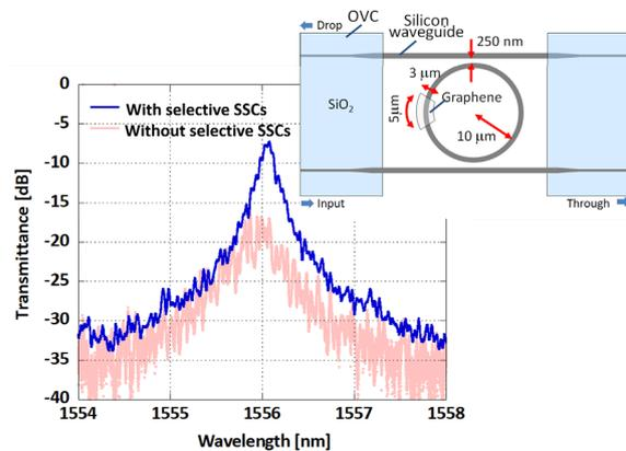
Fig. 4: Comparison of graphene integrated silicon-ring resonators for suppression of ripples, and inset is the schematic.
