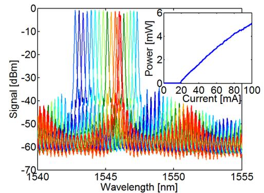
Fig.3: Typical spectrum when 40 mA are injected in both cavities. The phase sections are tuned by current injection. Inset shows a L-I curve obtained with a lensed fiber
