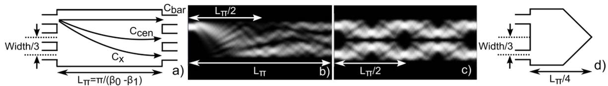
Fig. 2: (a) 2x2 MMI geometry. BPM simulation of (b) Single input excitation of MMI, (c) Anti-resonant excitation of MMI. (d) Related MIR geometry.
