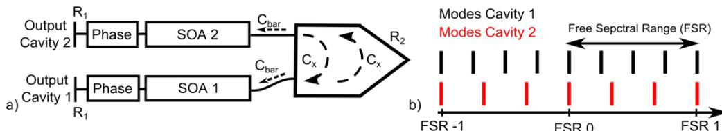
Fig. 1: Schematic of the Coupled Cavity Laser (CCL) (a) with indication of the tuning mechanism (b)
