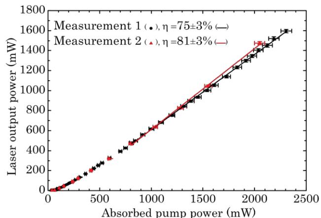
Fig. 1: Laser output power at 1840 nm versus absorbed pumped power at 794 nm in TM-polarization. Shown are two independent measurements (red and black dots), and the linear fits of the laser slope efficiency at higher powers (red and black lines).
