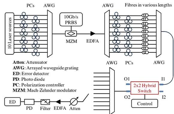
Fig. 2: Schematic of the experimental test-bed.
