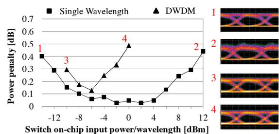
Fig. 4: IPDR curves for both single wavelength and DWDM operation eye diagrams shown for the numbered operating points.
