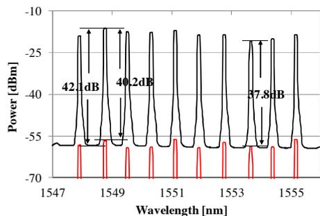
Fig. 3: Crosstalk measurement of 10 channels (the upper black curves represent the routed signal, while the lower red show the crosstalk signal).
