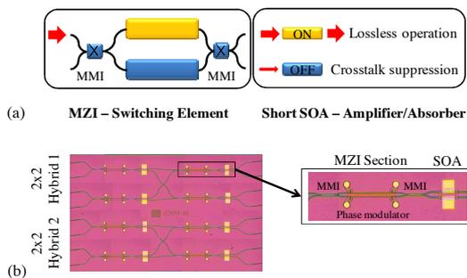
Fig. 1: (a) Schematic of operating principle. (b) Photograph of the fabricated hybrid switch.
