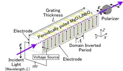
Fig. 1: EO polarization conversion type modulator using PPMgLN.
