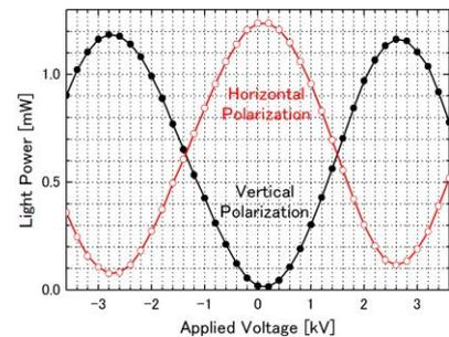
(b) Input: Horizontal polarization
