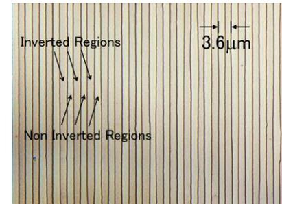
Fig. 2: Fabricated domain-inverted structures after etching.
