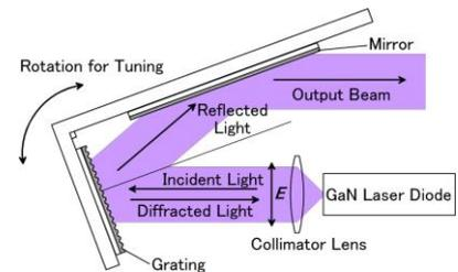
Fig. 3: Complex resonator laser using external grating.
