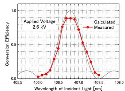
Fig. 6: Dependence of conversion efficiency upon wavelength. (Input: Vertically polarized light)
