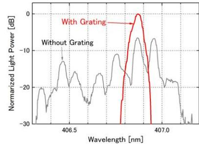
Fig. 4: Comparison of oscillation spectra. (Resolution: 0.04nm)
