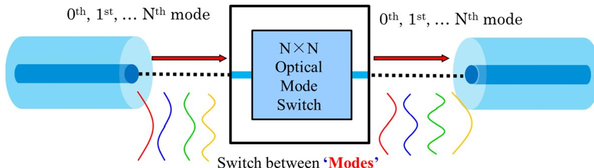
*Fig. 1: Schematic configuration of optical mode switch module.*
