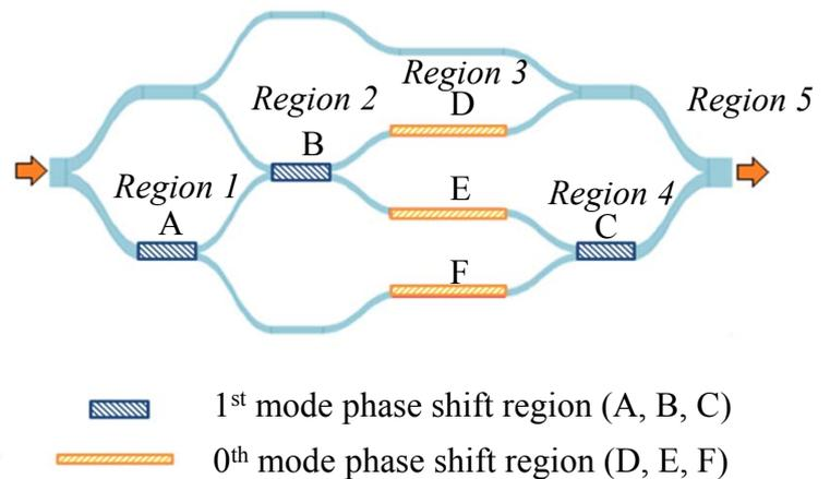
Fig.3: Schematic configuration of four mode optical mode switch.
