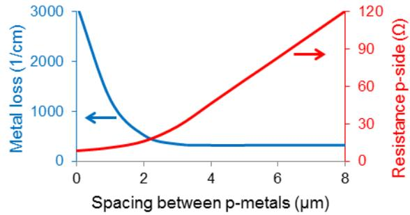
Fig. 3: Trade-off between metal loss and resistance.
