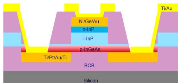
Fig. 1: Cross-section of the UTC-PD.
