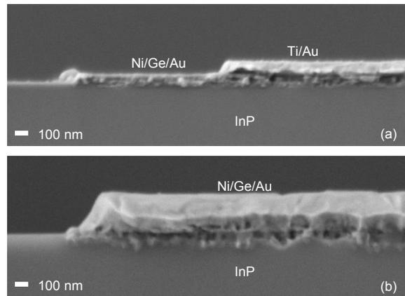
Fig. 4: SEM pictures of cleaved cross-sections.
