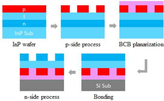
Fig. 2: Overview of double-side process.
