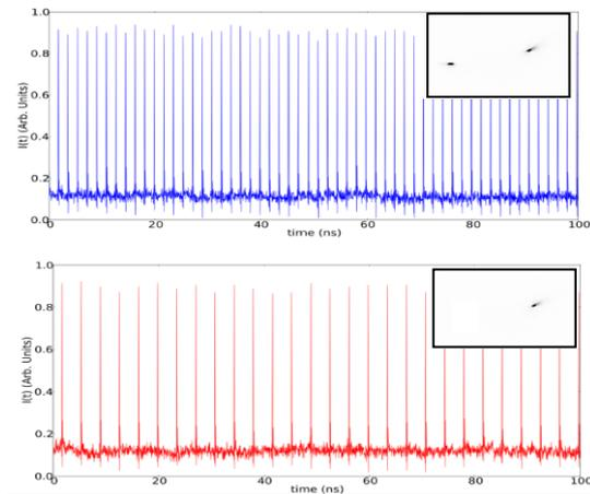
*Fig.3 upper panel: Intensity output from the VCSEL obtained when detecting the two spots of the far-field emission (inset) of the VCSEL. Lower panel: Intensity output from the VCSEL obtained when detecting only one spot of the far-field emission (inset) of the VCSEL.*
