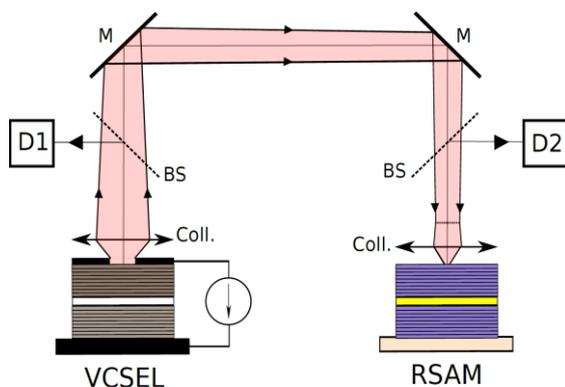
Fig.1: Experimental setup. Temperature stabilized VCSEL and RSAM. Coll : aspheric lens, BS: Beam Splitter, M : Mirror
