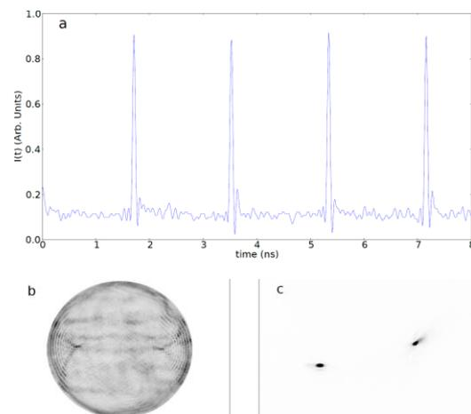
Fig. 2 : a) Total intensity output from the VCSEL in the mode-locking regime, b) near-field profile of the VCSEL, c) far-field profile of the VCSEL
