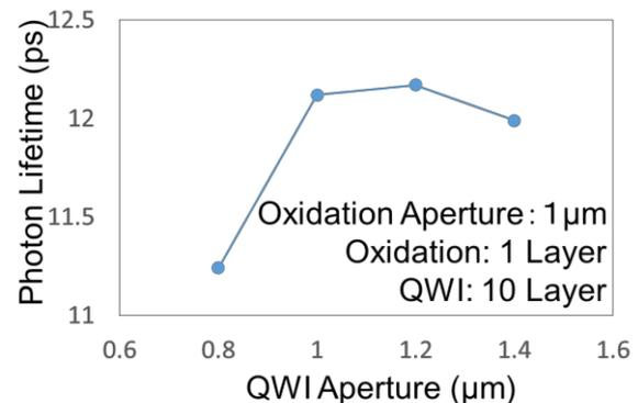
Fig. 4 QWI aperture dependence of photon lifetime.
