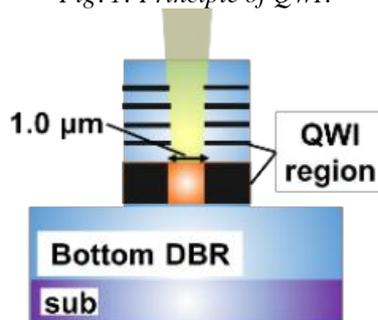
selective oxidation layer for the purpose of current confinement. In this study, the target aperture diameter of the QWI and the oxidation area is 1  $\mu\text{m}$ . The cavity loss was analyzed as photon lifetime, from the time decay of the light intensity using the two-dimensional FDTD.
