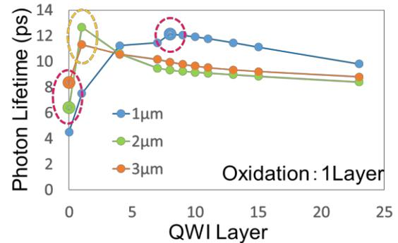
Fig. 3 Photon lifetime dependence on the QWI layer in DBR.
