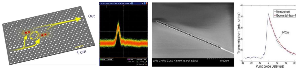
Fig. 2: On the left: layout of the two coupled H0 cavities forming the PhC "molecule" AOG and (center-left) response to a single short pulse in non-degenerate pump-probe measurement of the nonlinear dynamics. Center-right: two-port AOG based on a hybrid III-V PhC nanobeam cavity on a (SOI) waveguide and switch demonstration on a degenerate pump-probe experiment (on the right).
