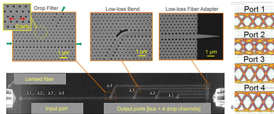
Fig. 1 Image of the 4-channel WDM demultiplexer (left) with magnifications of the resonant cavity, low-loss bend and fiber adapter. Eye diagrams of 100 Gbit/s signal after demultiplexing into 4x25 Gbit/s signals (right).
