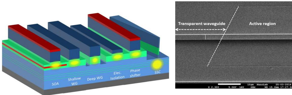
Fig. 3- (Left) Schematic of the building blocks in the long wavelength platform. From left to right, the following components are distinguishable: semiconductor optical amplifier, shallow waveguide, deep waveguide, electrical isolation, phase shifter and laterally-tapered spot-size converter. (right) top view of the junction between active and passive.
