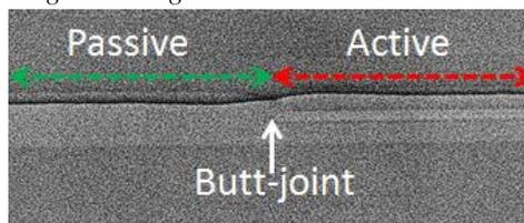
Fig. 2: SEM image of a cross-section through an active-passive butt-joint.
