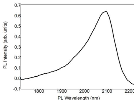
Fig. 1- Photoluminescence spectrum of the long-wavelength active material.
