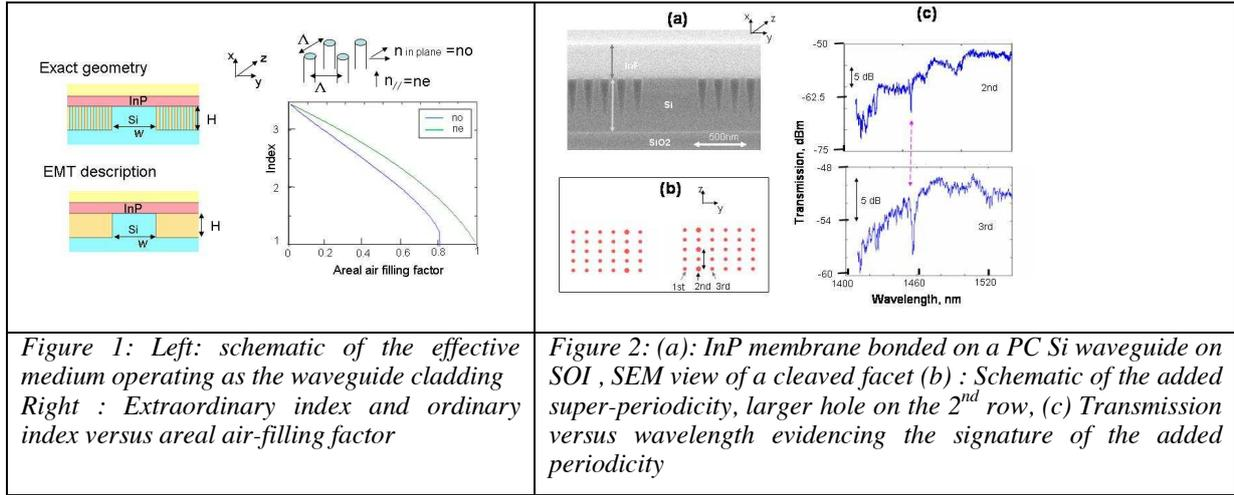
Figure 1: Left: schematic of the effective medium operating as the waveguide cladding Right : Extraordinary index and ordinary index versus areal air-filling factor
