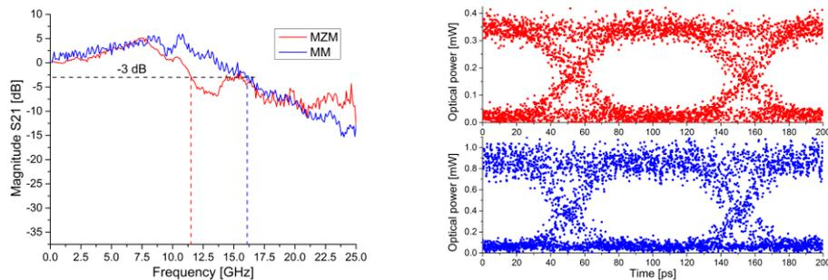
Fig. 3. Frequency response (left) and eye diagrams for an NRZ 10 Gb/s signal (right)
