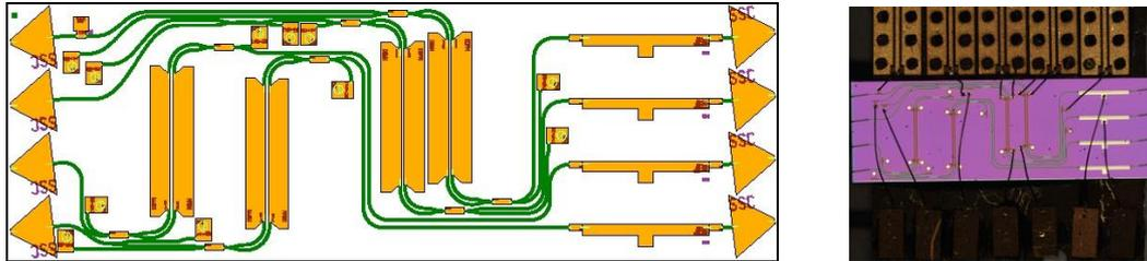
Fig. 2. Mask layout of the transceiver circuits in a transmitting configuration (left) and microscope photograph of the chip mounted for RF-characterization (right)
