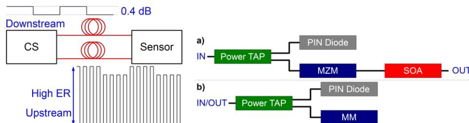
Fig. 1. Optical fiber link between the central station (CS) and a single sensor (left) transceiver circuit schemes in transmitting (a) and reflecting (b) configurations (right)
