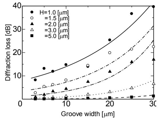
Fig. 2. Calculated diffraction loss depending on groove width.
