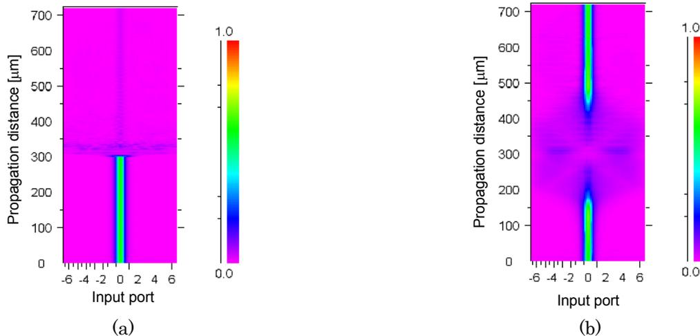
Fig. 3. Propagation characteristics of the TE mode (a) without a spot-size converter and (b) with a spot-size converter covered by a SiO<sub>2</sub> cladding layer.
