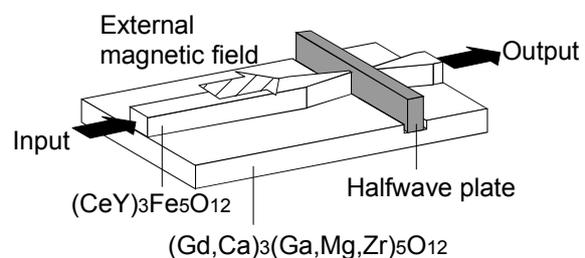
*Fig. 1. TE-TM mode conversion optical isolator with Ce:YIG guiding layer.*
