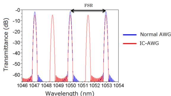
Fig.1: Transmission spectra of an IC-AWGR and a normal AWGR.
