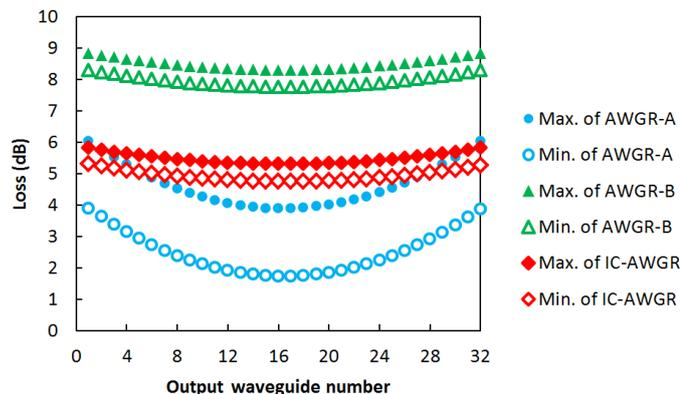
Fig. 2: Loss characteristics of AWGRs.
