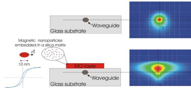
Fig. 1: Hybrid magneto-optic mode converter
