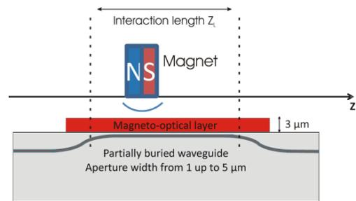
Fig. 2: partially buried waveguide
