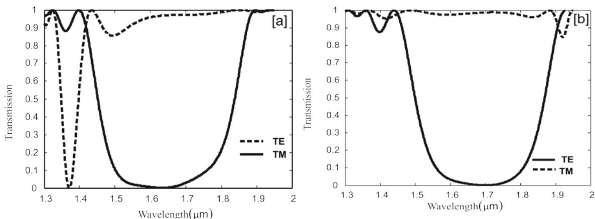
Fig. 1: Transmission spectra of designed polarization filters (a) TE-pass, (b) TM-pass.
