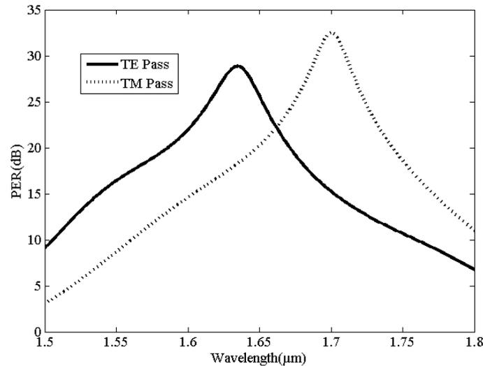
Fig. 2: Polarization Extinction Ratio for TE and TM Pass filters
