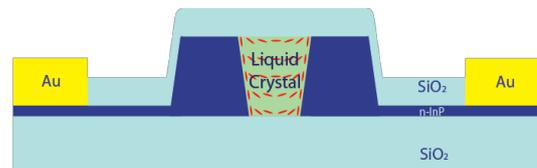
Fig. 1: Schematic of the phase shifter
