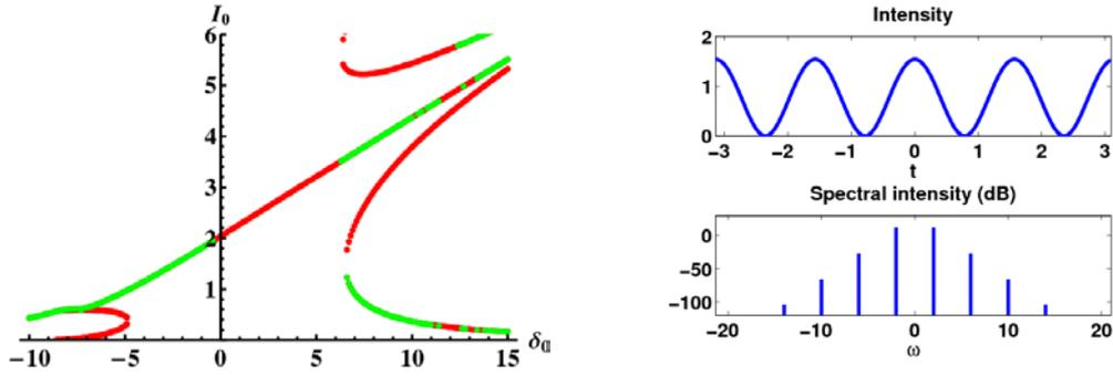
Fig.1: (left): Pump mode intensity  $I_0$  vs. detuning  $\delta_0$ , for  $\kappa = \beta\Omega^2 = -1$  and  $|f_0|=9$ . Green (red) curves indicate stable (unstable) intensities; (right): normal dispersion, background-free primary frequency comb.
