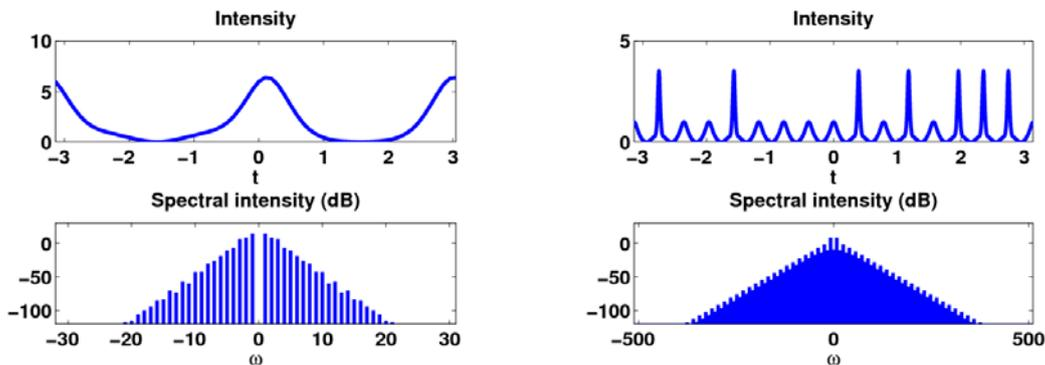
Fig.2: (left): Stable anomalous dispersion frequency comb without a background component but with even modes filled in due to secondary comb generation; (right): Coexistence of multiple injected cavity solitons on top of a stationary 16-bit pattern of low-intensity clock pulses.
