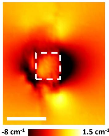
**Figure 1.-** Typical fluorescence image (in terms of spectral induced displacements) corresponding to a step-index Nd:YAG ceramic buried channel waveguides fabricated by direct laser writing. Scale bar is 10  $\mu\text{m}$ .
