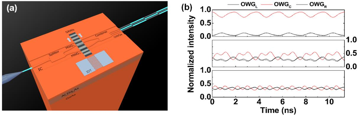
Fig. 1. (a) Illustration (not to scale) of the SAW-driven Mach-Zehnder interferometer with three output waveguides, fabricated on (Al,Ga)As. (b) Time-resolved traces recorded for the light leaving the OWG<sub>L</sub> (dotted black line), OWG<sub>C</sub> (solid red line) and OWG<sub>R</sub> (solid black line), measured for the TE polarization and RF powers of  $P_{\text{IDT}} = 6.8$  mW (upper panel),  $P_{\text{IDT}} = 68.3$  mW (central panel), and  $P_{\text{IDT}} = 108.3$  mW (bottom panel).
