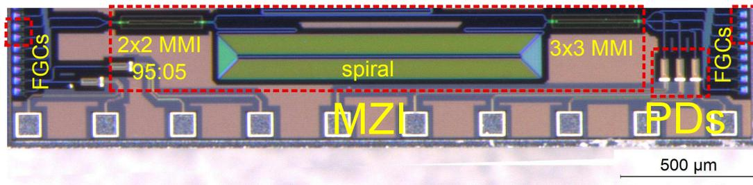
(a) Optical microscope image of the fabricated devices
