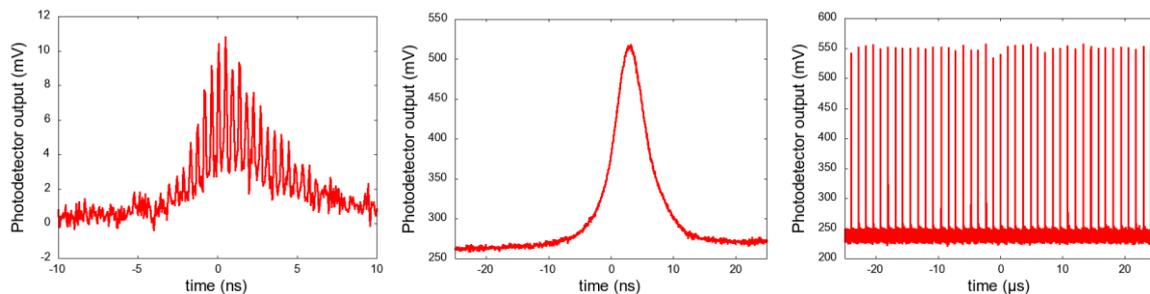
Figure 2: temporal characteristics of lasers. a): device A exhibits a Q-switched mode-locked operation. b) and c): device B is purely Q-switched.
