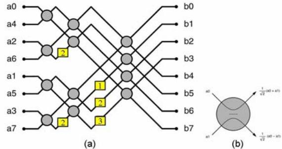
Figure 1. From [4]: (a) meshed fiber network composed of asymmetric couplers and phase shifters that performs the DFT of a parallel input. The phase shifters are represented by the boxes of value  $-q2\pi/N$  ( $q$  is the number inside the box). (b) asymmetric coupler.
