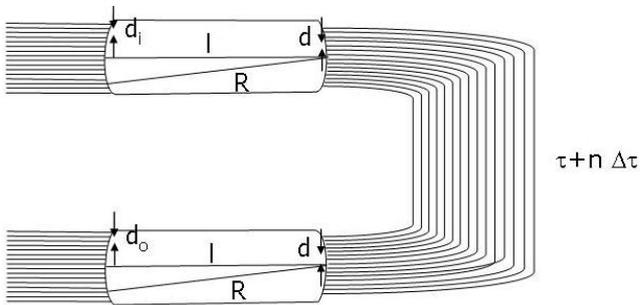
Figure 3. AWG architecture that performs the DFT.
