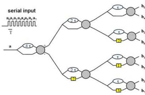
Figure 2. From [6]: tree architecture composed of MZIs with asymmetric couplers and phase shifters that performs the DFT of a serial input. The phase shifters are represented by the boxes of value  $-q2\pi/N$  ( $q$  is the number inside the box).
