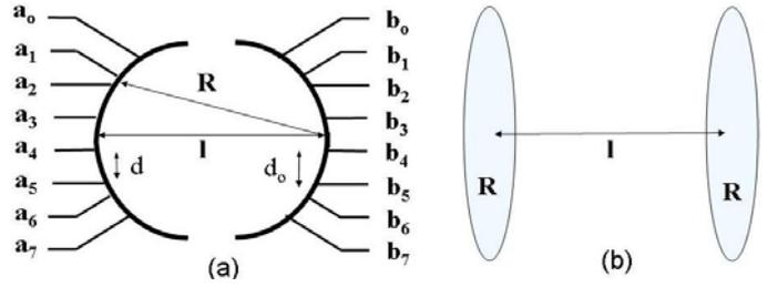
Figure 4. (a) slab coupler configuration. (b) two lenses configuration.
