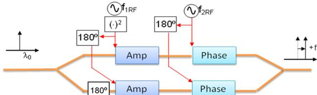
**Fig 1:** Functional description of the application-specific optical integrated circuit for wavelength shifting based in a Mach-Zehnder modulator, also showing the driving signals for the phase and amplitude (Amp) modulators.
