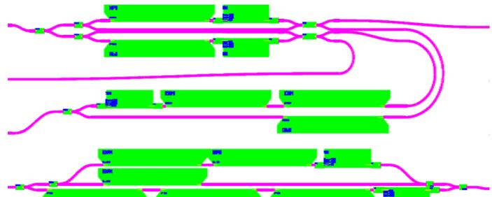
**Fig 3:** GDS view of the dual-arm (top) and triple-arm (bottom) wavelength shifter corresponding to the functional descriptions of Fig 1 and Fig 2.
