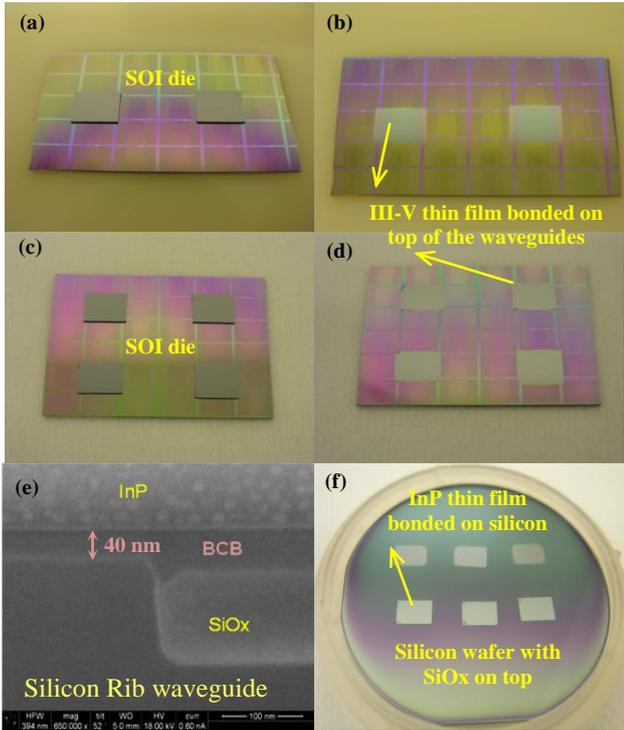
Figure 1. (a-b) two epitaxial  $0.3\text{ cm}^2$  III-V dies bonded on a planarized SOI die before and after the substrate removal process; (c-d) four epitaxial  $0.3\text{ cm}^2$  III-V dies bonded on a planarized SOI die before and after the substrate removal process; (e) SEM image of the bonding interface. (f) 6 InP-membranes (with the individual die area of  $0.2\text{ cm}^2$ ) bonded on a 50 mm silicon wafer.
