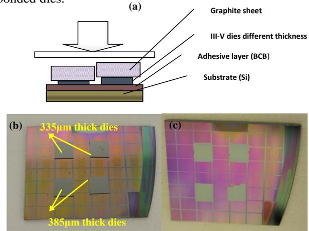
Figure 2. Bonding of four III-V dies, with different substrate thickness, on a planarized SOI die, using a graphite foil to compensate for the die thickness variations: (a) schematic; (b) before substrate removal; (c) after substrate removal.
