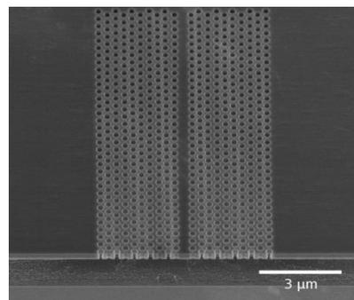
Figure 1. A scanning electron microscope image of a PhC WG.
