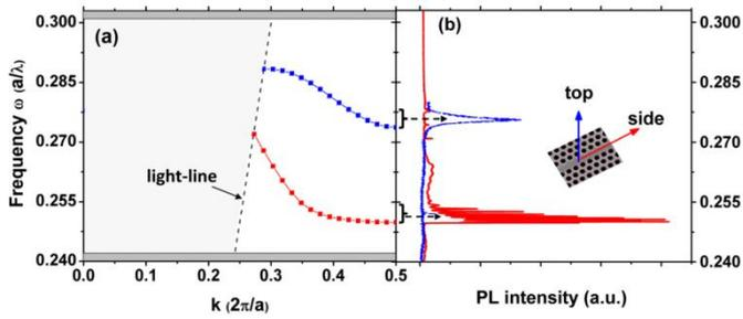
Figure 2. (a) Calculated band diagram and (b) PL data of a W1 PhC WG.
