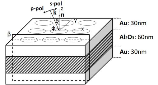
Fig. 1: Schematic of the MIM structure consisting of an Al<sub>2</sub>O<sub>3</sub> dielectric layer between two Au films perforated with a square array of elliptical holes suspended in air. The displacement current is shown in the plane  $\beta$
