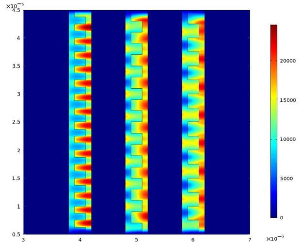
Figure 3. Absorption maps of 2D interdigitated organic solar cells for a wavelength of 450 nm. The inter-digit distances are 250 nm (left), 400 nm (center) and 500 nm (right). The units of the axes are microns.
