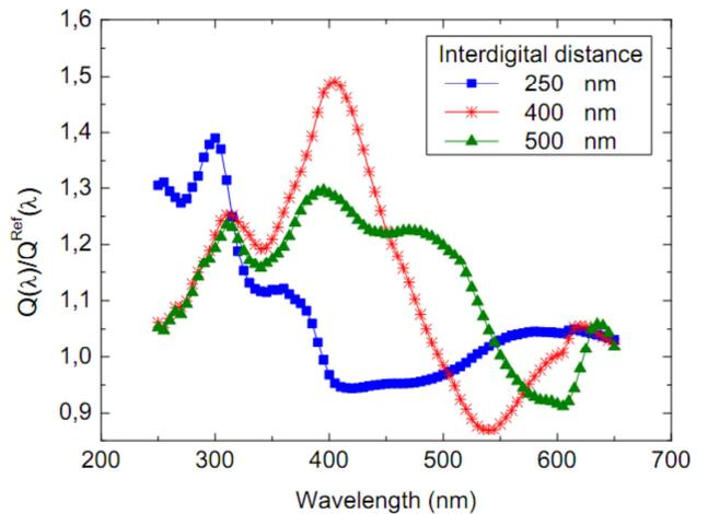
Figure 4. Spectrum of total absorbed energy of the interdigitated organic solar cells with respect to the total absorbed energy by a planar bilayer cell with the same amount of material.
