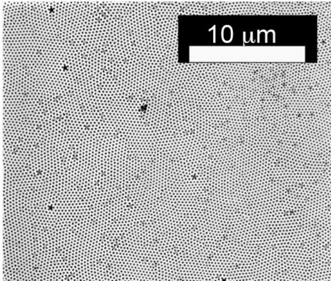
Figure 1. Example of a typical quasi-random nanoporous anodic alumina structure
