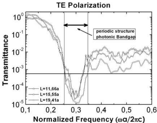
Figure 2. Transmittance in direction normal to the pores of a nanoporous anodic alumina. The minimum in transmittance appears at the same wavelength range than the photonic bandgap in a periodic structure with lattice constant equal to the average interpore distance  $a$ .
