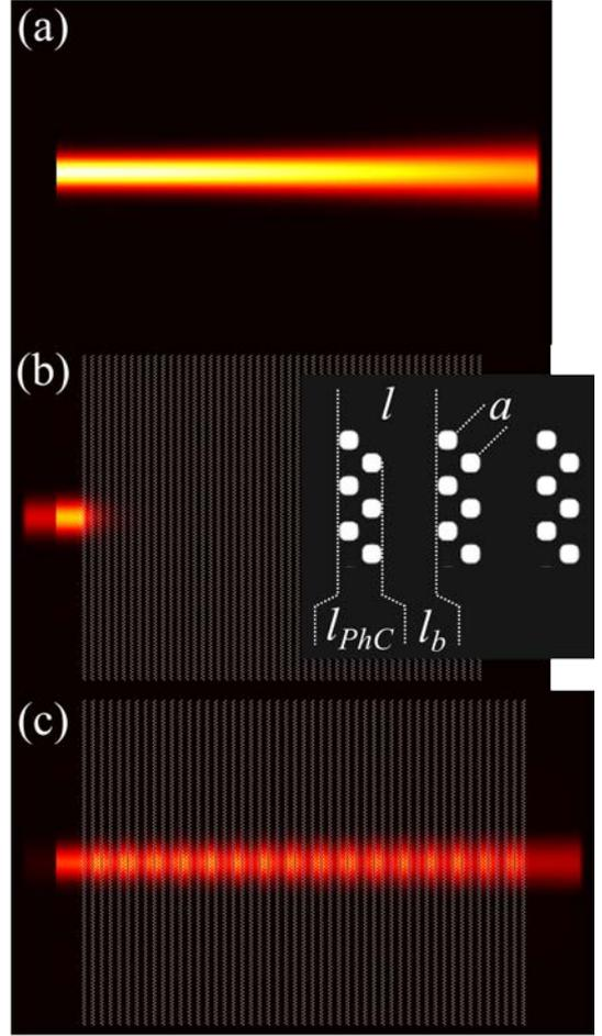
Figure 2. Energy distribution for a) reference raw material, b) DBR ( $a_{DBR}=448$  nm,  $l_b=1.156a\sqrt{2}$ ) and c) AR ( $a_{AR}=452$  nm,  $l_b=1.396a\sqrt{2}$ ) schemes.
