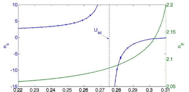
Figure 1. Phase index and curvature index of the first band versus the normalized frequency for the single-hole unit cell of an infinite 2D PhC ( $a/r=0.28$ ); dashed line corresponds to self-collimation ( $U_{sc}\sim 0.2754$ ).
