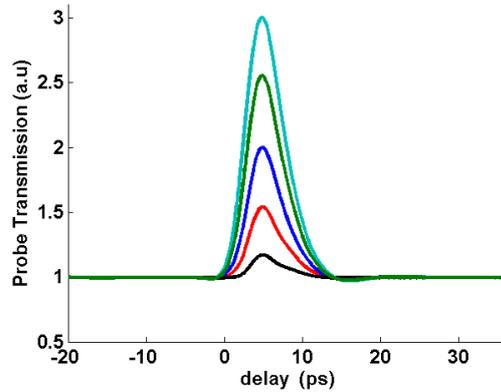
**Fig.2:** FDTD probe transmission for increasing values of the pump power density in a pump-probe configuration.
