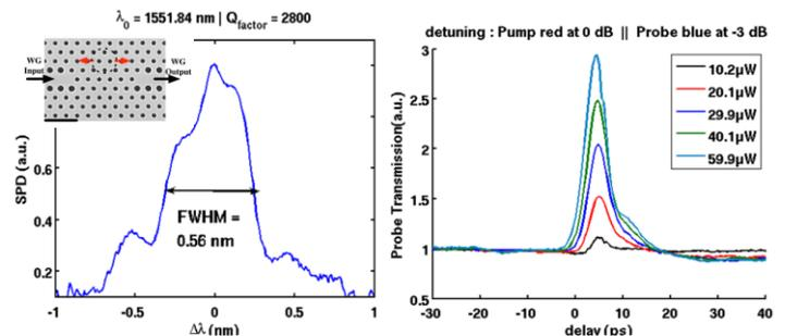
**Fig. 1:** Spectral response of the GaAs H0 nano-cavity (left) and time-resolved dynamics of the probe transmission (right). Switching is obtained in pump-probe configuration with the pump on resonance and the probe blue-shifted at -3 dB point of the spectral response.
