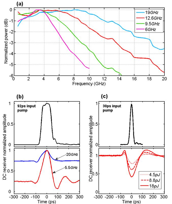
Figure 2. (a) Small-signal modulation response of converted probe for various probe fringes. (b) and (c) Pump and probes transmission dynamics of a single 92 ps and 30 ps wide pulse, respectively.
