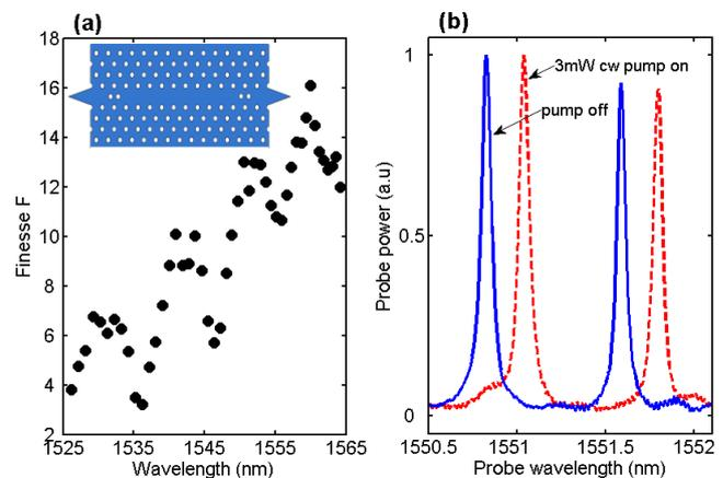
Figure 1. (a) Finesse spectrum of the resonator. Inset: Structure of the resonator. (b) Static transmission spectrum: pump off (blue) and on (red).
