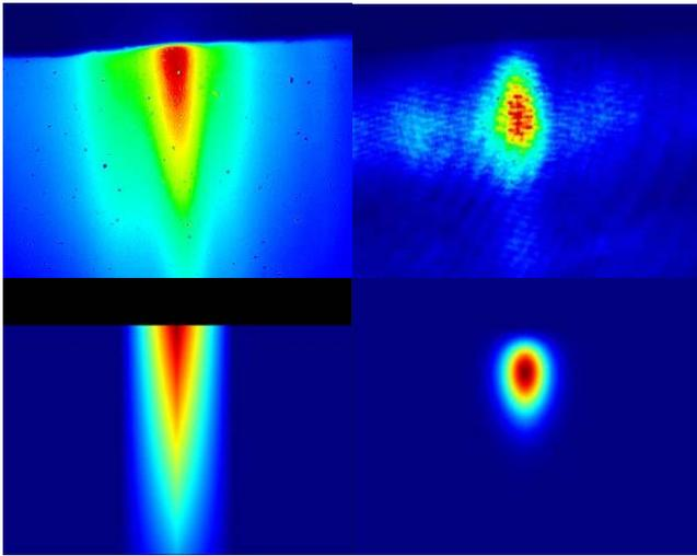
Figure 2. (a) Measured 1000nm+ luminescence due to pumping. (b) Measured guided He-Ne mode profile. (c) Reconstructed refractive index profile chosen to match luminescence. (d) Reconstructed mode profile by optimising the magnitude of refractive index change in c. Individual images sizes are width=153 $\mu$ m, height =123 $\mu$ m.
