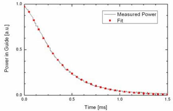
Figure 3. He-Ne power in waveguide after switch off of the diode-laser pump. This power has been shown to be proportional to the refractive index change of the waveguide due to the small index change and large coupling angle. Overlaid is a fit using equation 2.
