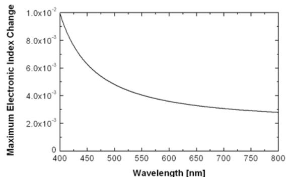
Figure 1. Maximum electronic refractive index change in KYbW assuming 50% of Yb<sup>3+</sup> ions are excited into the <sup>2</sup>F<sub>7/2</sub> energy level for a range of wavelengths for which the crystal is transparent.
