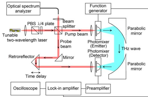
Figure 2. Experimental setup for coherent THz wave generation and detection using tunable two-wavelength laser and two photomixers.
