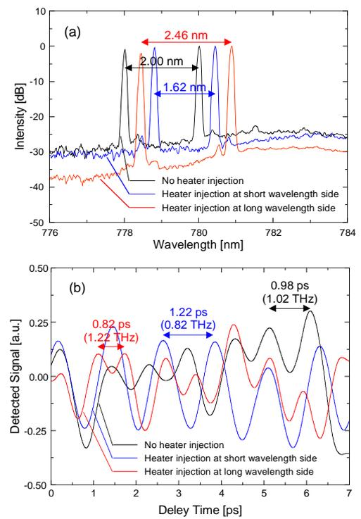
Figure 3. (a) Measured spectra of tunable two-wavelength oscillation, and (b) dependence of detected signals on delay time.
