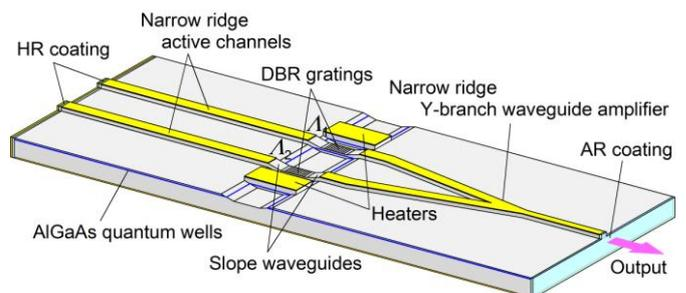
Figure 1. Schematic of integrated tunable two-wavelength DBR laser.
