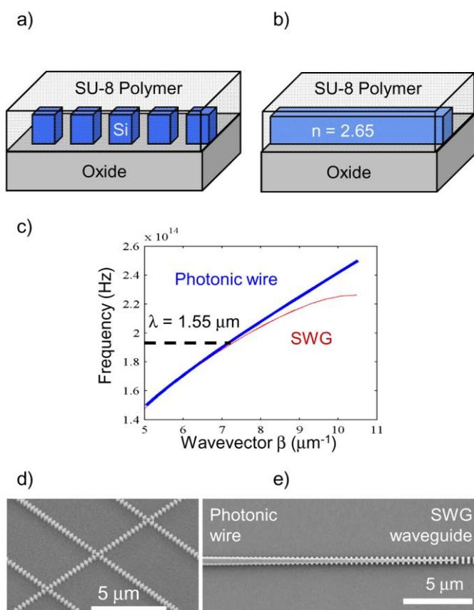
Fig. 1 a) Schematic of a silicon SWG waveguide. b) Equivalent wire waveguide with spatially averaged core index. c) Comparison of the calculated dispersion diagrams of the structures shown in a) and b). d) Scanning electron micrograph (SEM) of SWG waveguide crossings. e) SEM of low-loss SWG fiber-chip coupling structure.
