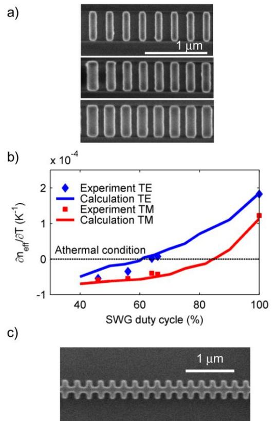
Fig. 2 a) SEM micrographs of SWG waveguides with Si duty ratios of 46%, 56% and 66%. b) Experimental and theoretical results for the effective thermo-optic coefficient of SU-8 clad silicon SWG waveguides as a function of grating duty cycle. c) SEM of a SWSG waveguide.
