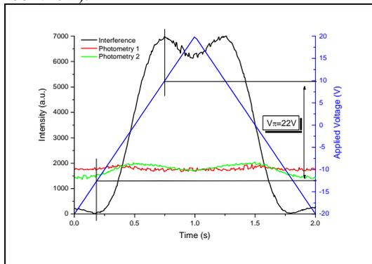
Figure 2. Modulation achieved in the combiner, using monochromatic laser light and a 40Vpp triangular ramp.
