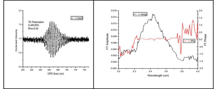
Figure 3. Left: TE wide band fringes. Right: Amplitude and Phase of the Fourier Transform of the wide band fringes.
