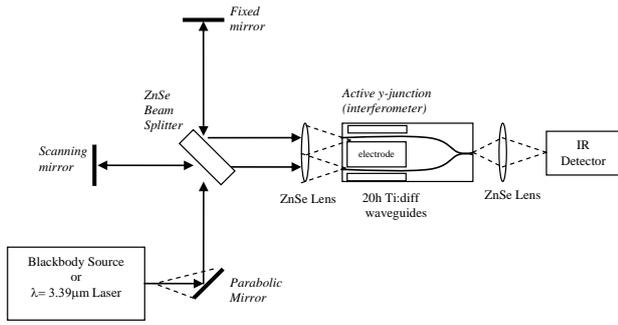
Figure 1. Schematics of the experimental set-up allowing intensity modulation in the mid-IR.
