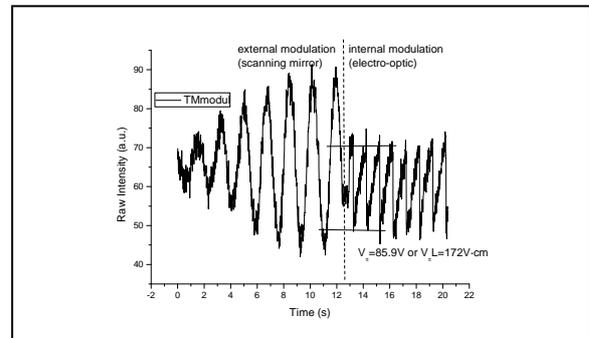
Figure 4. Electro-optic modulation of the wide band fringes in TM polarization. Note that below 13s the fringes are scanned externally.
