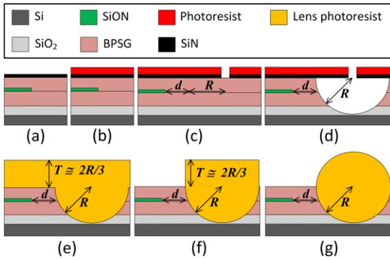
Figure 2. Process flow of microlens fabrication on pre-existing waveguide structure. (a) SiN deposition, (b) Spinning of photoresist and mask exposure, (c) development of photoresist and etching of SiN, (d) Isotropic etch of BPSG through buffered hydrofluoric acid (BHF) to achieve a semi-sphere with radius  $R$ , (e) Spinning of lens photoresist with height  $T \approx 2R/3$ , (f) Exposure and development of resist using the lens mask, (g) reflow of resist at  $\sim 130$  °C.
