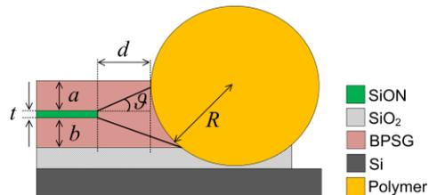
Figure 1. Schematic of microlens, where  $t$  is the thickness of the SiON layer,  $a$  and  $b$  are the thicknesses of the upper and lower BPSG claddings,  $d$  is the distance of the micro-lens from the waveguide facet,  $R$  is the lens radius, and  $\theta$  is the angular aperture of the waveguide inside the BPSG.
