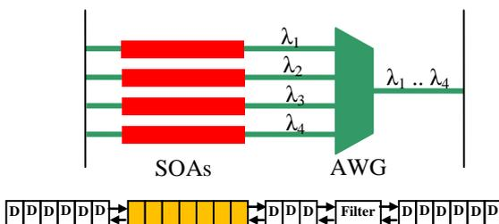
Figure 1. Schematic of an AWGL and equivalent model.
