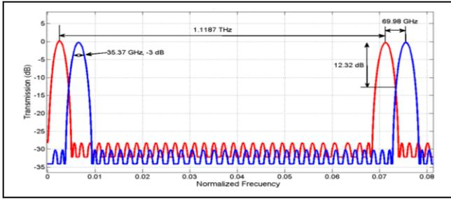
Figure 3. Matlab AWG equivalent digital filter response.
