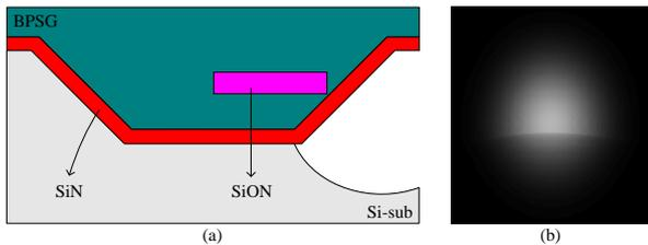
Figure 2. (a) Cross-section of the simplified mirror structure used in the simulation and (b) calculated far field intensity profile.
