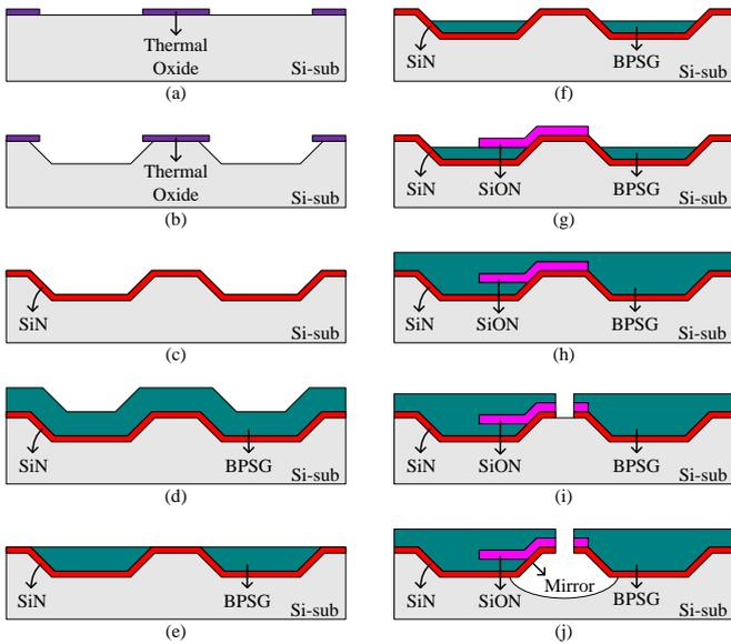
Figure 1. Wafer cross-sections corresponding to different steps in the fabrication process flow.
