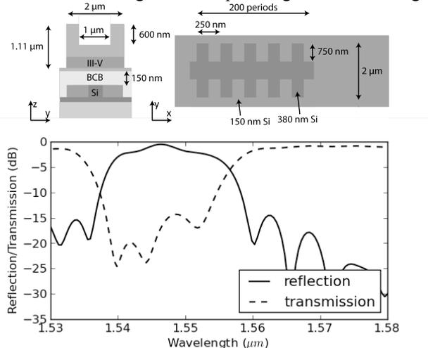
**Figure 2: Reflection and transmission spectrum of proposed resonant mirror**
