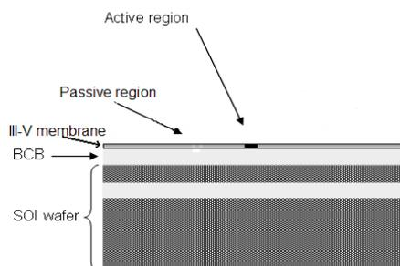
Figure 1. The layer stack of the IMOS platform
