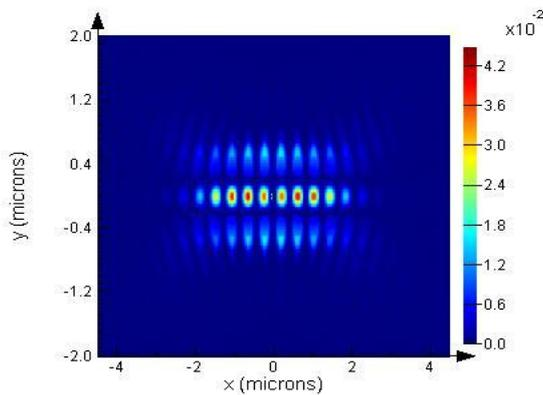
Figure 4. Mode field profile of the main resonant mode
