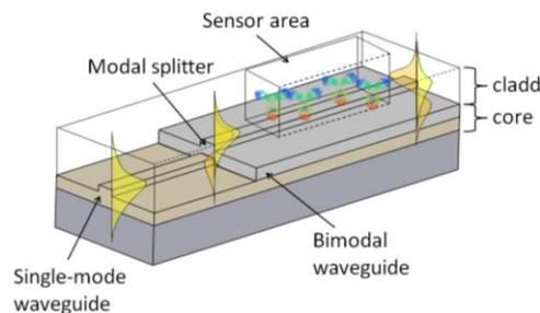
Figure 1. Scheme of a BiMW sensor.
