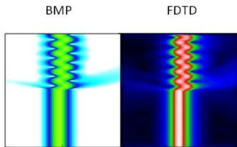
Figure 3. Logarithmic representations of the electromagnetic field in the splitter region of a BiMW device by BPM and FDTD methods.
