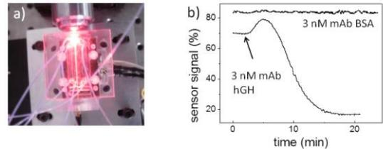
Figure 5. a) 4-channel fluidic cell and b) interferometric detection of a 3 nM of mAb hGH.
