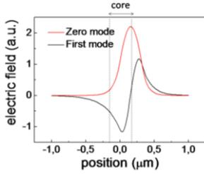
Figure 2. Distribution of the electric field of both modes in the bimodal waveguide.
