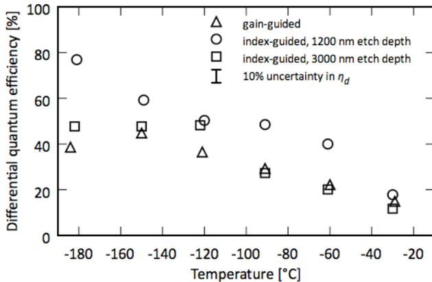
Figure 2. Differential quantum efficiency  $\eta_d$  plotted as a function of sample temperature for lasers with different etch depths, i.e. rib heights
