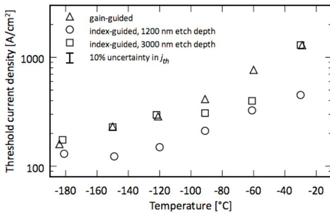
Figure 3. Threshold current density  $j_{th}$  plotted as a function of sample temperature for lasers with 1000  $\mu\text{m}$  long and 100  $\mu\text{m}$  wide active regions and different etch depths
