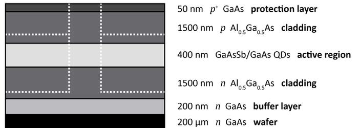
Figure 1. Laser layer design (not to scale). The white dotted lines denote the two etch depths / rib heights
