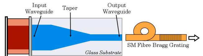
Figure 1. Fundamental mode locking and wavelength stabilization
