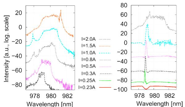
Figure 2. Emission spectrum of the solitary laser diode on the left and of the system on the right for different injection currents.
