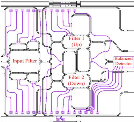
**Fig. 3:** Chip layout for the Chebyshev design.
