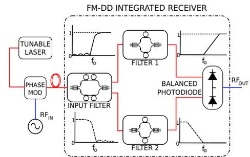
**Fig. 1:** Block diagram of the device. Optical power transfer functions at the output of each filter are shown.
