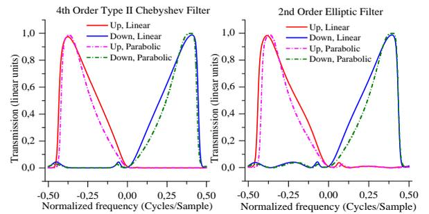
**Fig. 2:** Simulated transfer function of each input filter (Chebyshev & Elliptic), when combined with two different frequency discriminators (Linear & Parabolic).
