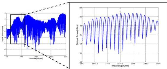
Figure 5: Measured spectral response at the DPSK demodulator. Inset: zoom in resonance of interest.
