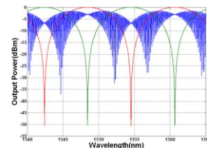
Figure 2 Simulated spectral response at the MZDI inputs (green, red) and at the demodulator output (blue).
