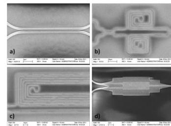
Figure 3: SEM images of a) 3dB Coupler, b) MZI with  $\Delta L=50\mu\text{m}$ , c) MZDI, d) 2x1 MMI
