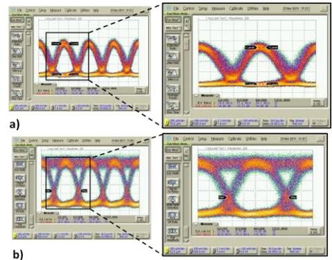
Figure 7: Eye diagram of the 20Gb/s-NRZ-DPSK for a) AMI and b) DB demodulated signals.
