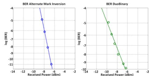
Figure 8: BER curves for based DPSK demodulation at 20 Gb/s operation for a) AMI and b) DB demodulated signals.
