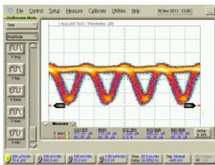
Figure 6: Eye diagram of the 20Gb/s-NRZ-DPSK input signal
