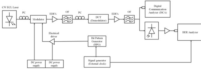
Figure 4: Block diagram of the experimental DPSK demodulation setup
