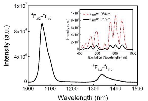
Figure 1. Infrared emission spectra in 5wt% Nd<sub>2</sub>O<sub>3</sub> doped NMAG glasses. Inset: Excitation spectra for 1.064 and 1.337  $\mu$ m emissions
