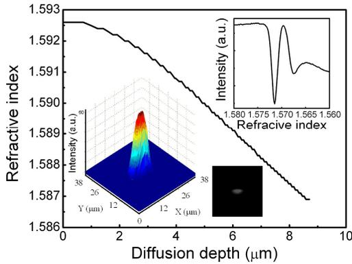
Figure 2. Index profile of a slab waveguide measured at 632.8nm. Upper inset: Prism coupler result measured at 1536nm. Bottom inset: Near-field mode pattern and a 3D representation of the channel waveguide at 1.3 $\mu$ m.
