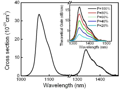
Figure 3. Stimulated emission cross-section profiles for the  ${}^4F_{3/2} \rightarrow {}^4I_{11/2}$  and  ${}^4F_{3/2} \rightarrow {}^4I_{13/2}$  transitions in 5wt% Nd<sup>3+</sup> doped NMAG glasses. Inset: Calculated theoretical gain spectra of the  ${}^4F_{3/2} \rightarrow {}^4I_{13/2}$  transition.
