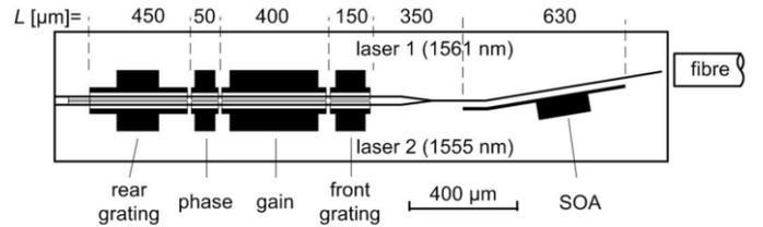
Figure 1: Schematic of the optical chip
