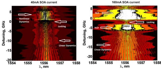
Figure 2: Optical maps for SMLs of -26 dB (lhs) and -11 dB (rhs).
