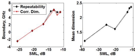
Figure 3: Modelled nonlinear trends as a function of FWM levels: 3a (lhs): frequency boundary linear-nonlinear behavior; 3b (rhs): overall degree of nonlinearity at low detuning (-5 GHz to +5 GHz).
