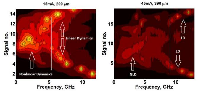
Figure 4: Experimental single-sided spectral maps for SMLs of -26 dB (lhs) and -16 dB (rhs). The vertical white lines show the boundaries between linear dynamics (LD) and NLD that were calculated using the correlation dimension of the time series.
