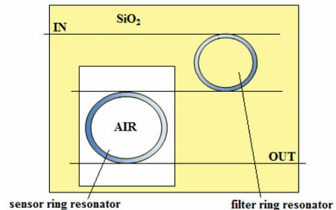
Figure 1. Architectural scheme of an integrated photonic sensor based on Vernier-effect in SOI technology, using a  $\text{SiO}_2$  insulating cladding.
