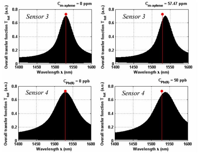
Figure 3. Simulations of *Sensor 3* and *Sensor 4* operation for m-xylene and lead Pb(II) detection. Red line is set at  $\lambda_{sensor} = 1529.4$  nm.
