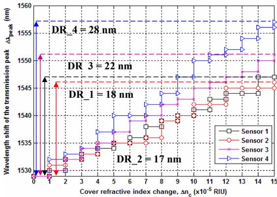
Figure 2. Wavelength shift  $\Delta\lambda_{peak}$  versus cover RI change,  $\Delta n_c \sim 10^{-5}$  RIU, for various selected sensing architectures.
