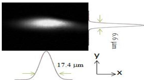
Figure 1. Near field fluorescence intensity for a waveguide etched by ion-beam milling in (Yb,Nb):RTP along with the x and y mode profiles.
