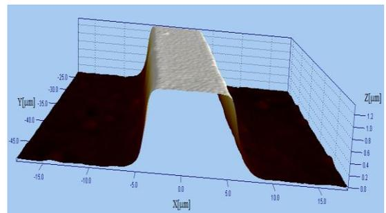
Figure 2. 3-d image of an RIE etched rib feature in RTP
